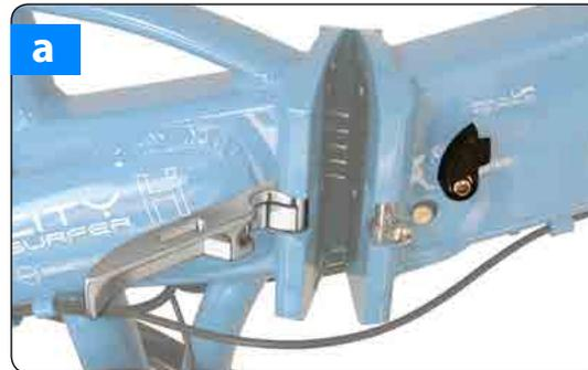
Folding the Citysurfer is very easy. The system to fold the bike is located on the central part of the frame, on the right side of it. Firstly, turn upwards the security black piece to unlock the folding lever. After that, pull outwards the silver lever. In this moment the frame is free to be folded in half\*.
