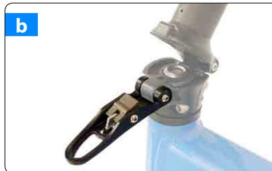
Push the secure close button located in the base of the steering shaft to fold the handlebar. Then pull downwards the lever and the handlebar will be released. Move the handlebar in the direction of the hinge to place it beside the wheel. The cables are designed to change their position without any problem.
