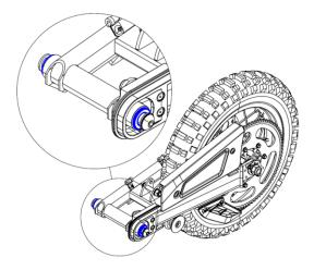
If the swingarm or its bushings show any kind of damage or signs of deterioration, they must be replaced.
