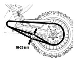
Rotate the rear wheel moving the tire with your hand, stopping at different positions to check the chain's clearance, always taking the measurements in the same place.
