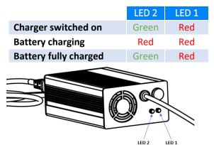
The LED 2 will turn green when the battery is fully charged. It will take about 4 hours to fully charge in the case of a series ONE battery, and 5.5 hours for a full charge in the case of a KIDS TWO series.
