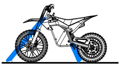
Then compress the forks and rear shock absorber before hard pulling the strips to fix the motorcycle.
