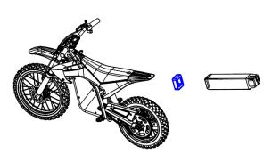
maximum capacity. To connect it for the first time, and after each ride, the battery must be removed as explained in the <u>Charge the battery outside the vehicle</u> section and the foam spacer that is between the battery connector and the battery compartment should be removed.
